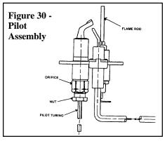
CAUTION: Due to high voltage on pilot spark wire and pilot electrode, do not touch when energized. See Hazard Levels, page 2.
